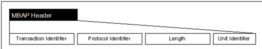
[Figure 5-4] Structure of Modbus TCP/IP ADU
