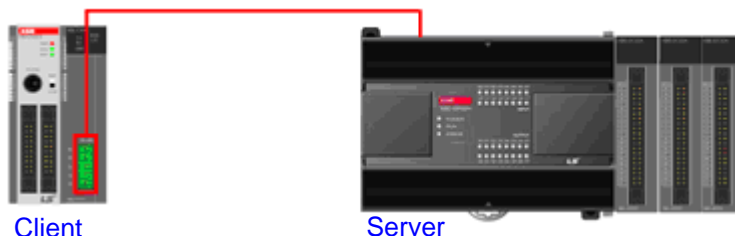
[Figure 8.3.1] XGT Modbus communication system configuration example
