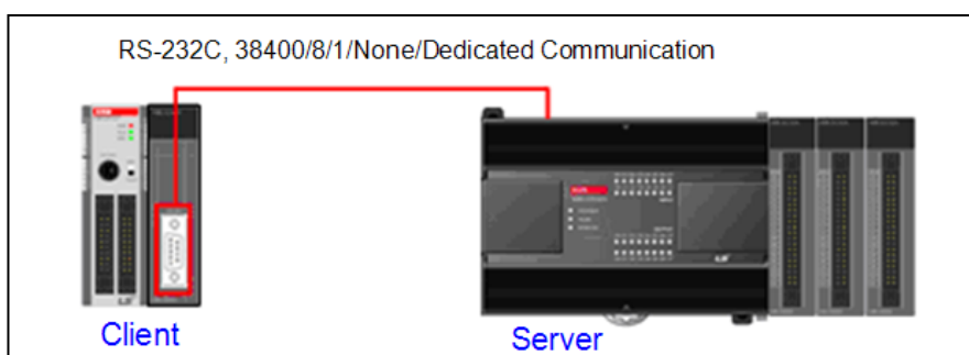
[Figure 8.2.1] Example of dedicated service system configuration
