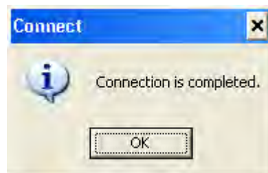
[Figure 12.1.11] Redundant CPU connection completed
