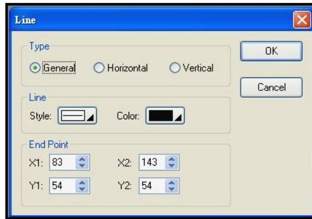
To change the length or the position of the lines, click the target line to see two checks at the ends of the line, move the cursor on the checks. After the cursor turns to a cross arrow, press the left button of the mouse and drag the line to any position you like on the working area.
