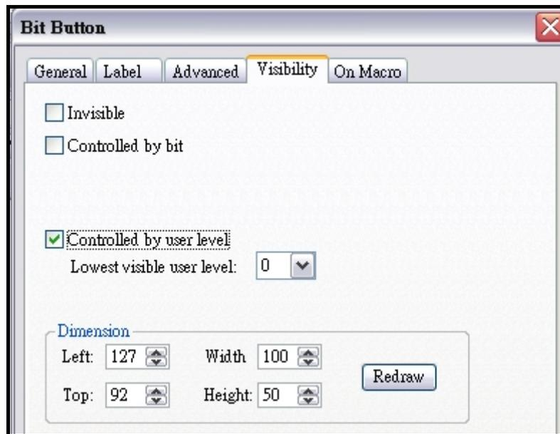
Figure 2-10 Object properties dialogue \_bit button visibility settings
