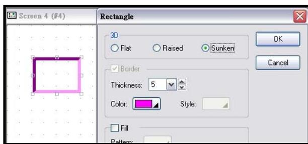
Click Sunken to select Thickness and Color. The Border is not selectable. When a color is chosen, PanelMaster shows default coordinated dark color on the left and top of the rectangle.
