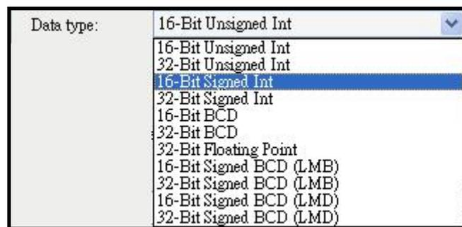
**Data Type** : There are several data format type, 16-bit unsigned int., 32-bit unsigned int., 16-bit signed int., 32-bit signed int., etc.. LMB express if left most bit as 1 then the value is negative. LMD express if left most digit (4 bits) as F then the value is negative.
