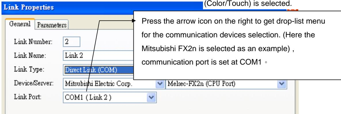
Link Name : Link1\_FX2n, when there is a communication error, the name of Link will show on the communication error screen.
