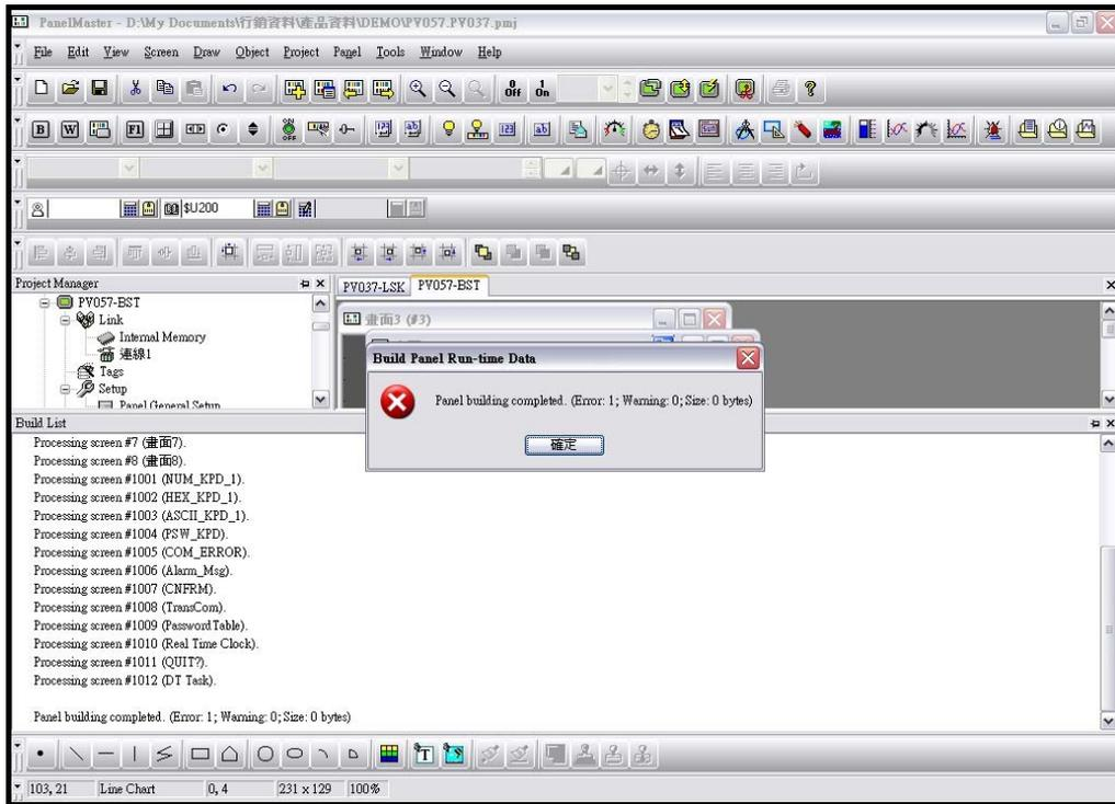
Figure 2-98 New project\_step 7\_ Build touch panel run-time data
