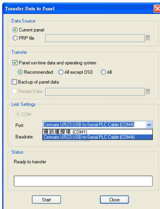
Figure 2-71 Panel menu\_ Transfer Data to Panel
