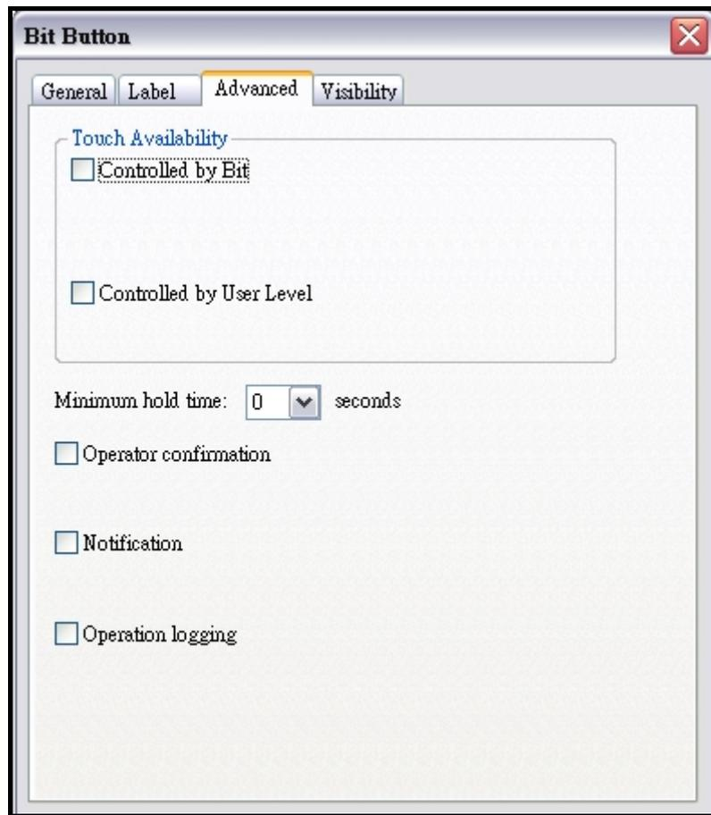
Figure 2-9 Object properties dialogue \_bit button advanced settings
