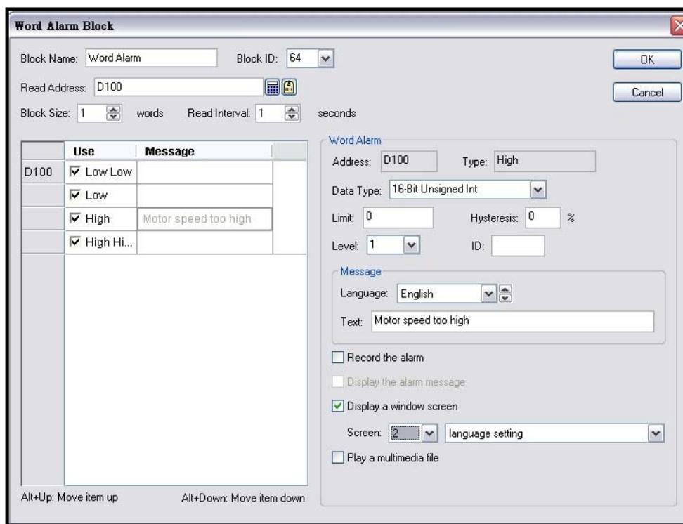
Figure 2-41 Object properties dialogue \_word alarm block
