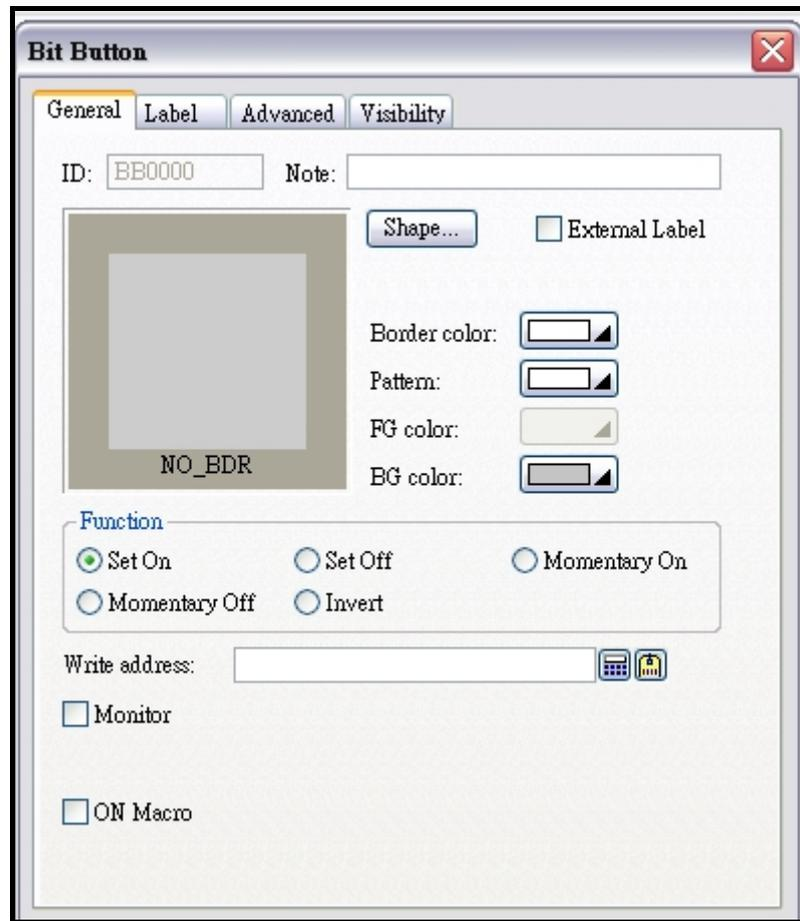
Figure 2-7 Object properties dialogue \_ bit button general setting
