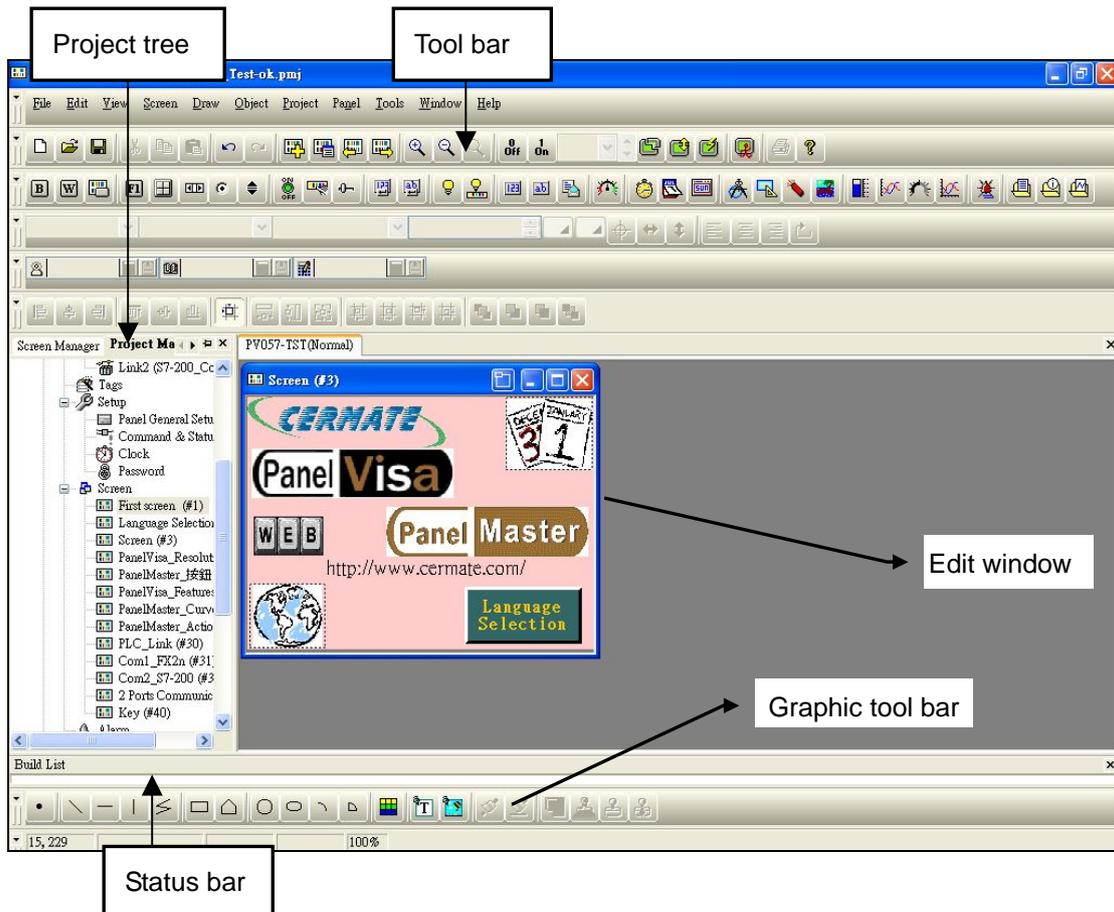
The project manager and screen manager tree are on the left side of the program screen. This area is for quick setting of the main functions and for overview.
