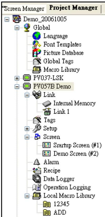
**Link** : Assign the devices the panel communicates to. There are Internal Memory · PLC IO or PLC data registers. PanelMaster supports Multi-link function that is the panel's serial ports link with different kinds of PLC.
