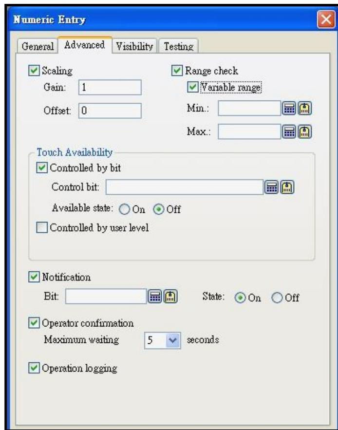
**Scaling:** Only when the 16-Bit Unsigned Decimal provides this function. The scaling formula is  $(Y=aX+b)$ .
