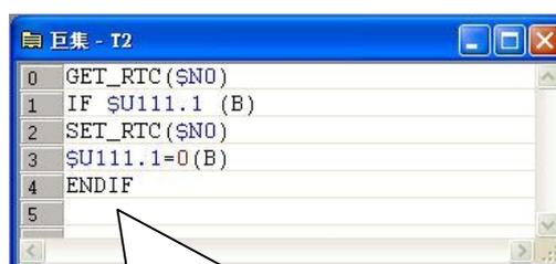
Use Macro instruction GET\_RTC to send RTC value to Register, and SET\_RTC will set the Register value to the RTC. This example uses HMI internal data register SN0.
