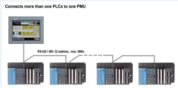
$^{\ast}$  1:N communication by using RS-422/485 should be organized as choosing identical PLC types
