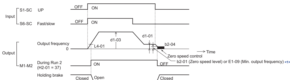
Figure 4.15 Holding Brake Time Chart (CLV, CLV/PM)
