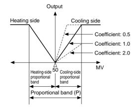
• When *P* is set to 0.0 and *Lool* is set to 0.0 in the dual output type, the cooling output is as shown in the figure below. The hysteresis is fixed at 0.5% FS.
