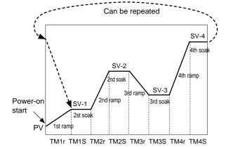
• The segment in which both the ramp time and soak time are set to "0" is skipped.
