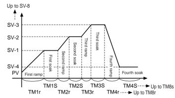
Ramp: the section in which the SV changes toward the target value. Soak: the section in which the SV is the target value, and remains unchanged.
