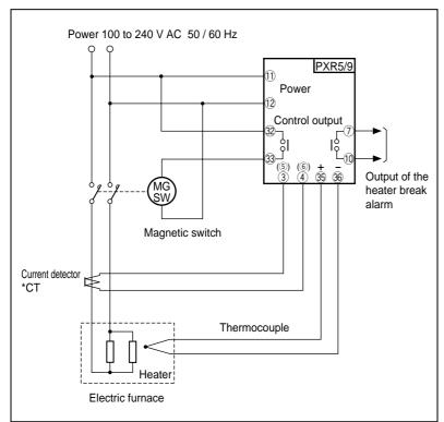
• Connection example for the alarm for heater break (PXR5/9 model)
